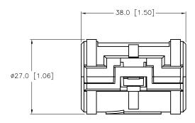
LOCKOUT DEVICE FITS STRAIGHT TURCK EUROFAST FIELD WIREABLE CONNECTORS B(S)(V)  $81\times1-0$  AND B(S)(V)  $81\times1-0/PG9$ ".
